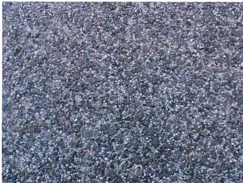
Picture 3: Surface texture of the asphalt surface course with hydrated lime
