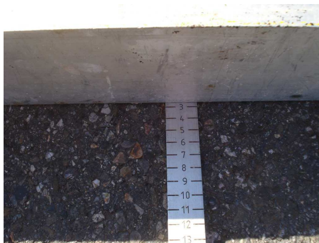
figure 5: ruts section B, L 181
