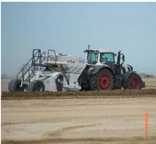
Figure 4.12 – Dosing and mixing chamber on same tractor-pulled soil stabiliser (© Carmeuse)
