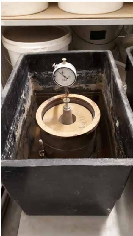
Figure 2.4 – Swelling measurement of CBR samples after 4 days' storage in water (© BRRC)
