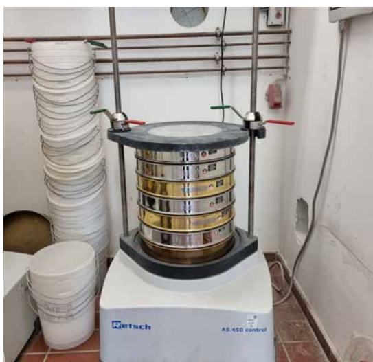
Figure A1.1 – Grading size equipment (© Federal Association of the German Lime Industry e.V.)
