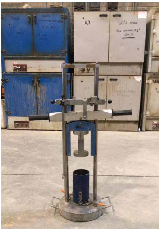
Figure 3.2 – MCV equipment (© Balfour Beatty, Major Projects Materials Department)
