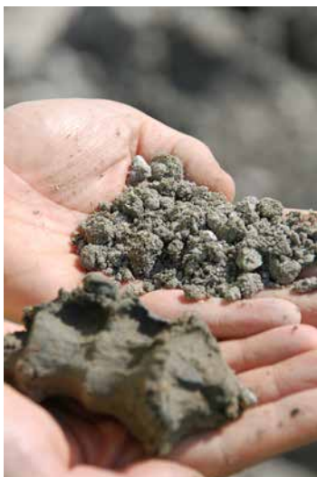
Figure 2.7 – Initial state and flocculated clay soil after lime addition (© Lhoist)
