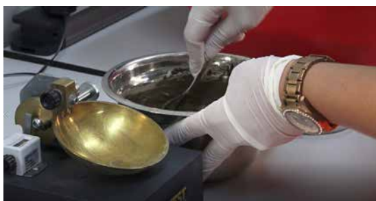
Figure A1.4 – Liquid limit test – Casagrande method (© Carmeuse)
