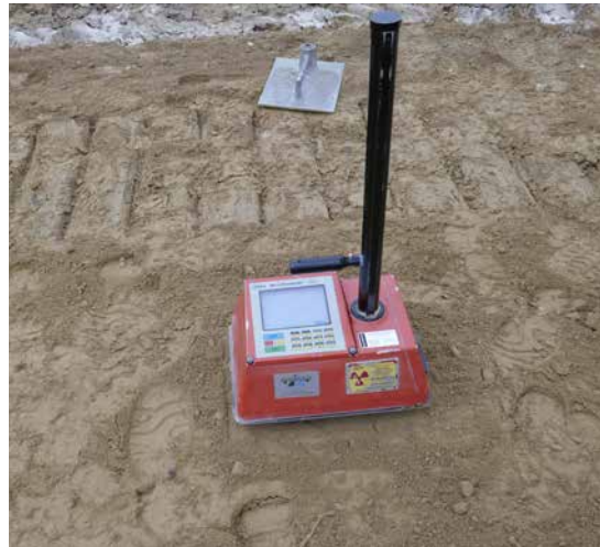
Figure 4.27 – Control of moisture, density, compaction ratio by nuclear gauge (© Carmeuse, BRRC)
