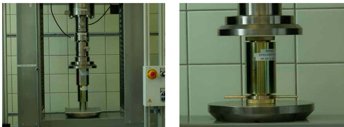
Figure 3.4 – Static compaction (© BRRC)
