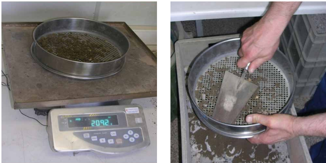
Figure A1.18 – Pulverisation test (© BRR)
