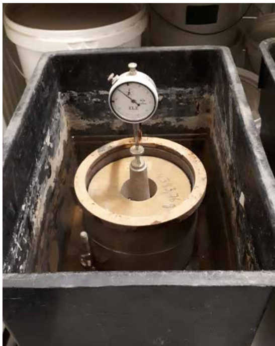
Figure A1.17 – Swelling test (© BRRC)
