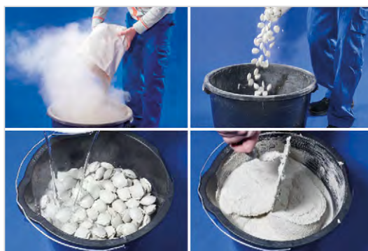
The preparation of traditional mortar (first photo) versus compact mortar pellets.
