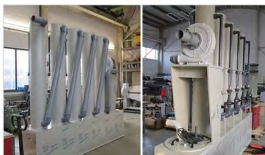
Pilot CO 2 scrubber of ECO 2 project, Wilhelmshaven coal-fired power plant, where pilot testing is carried out.
